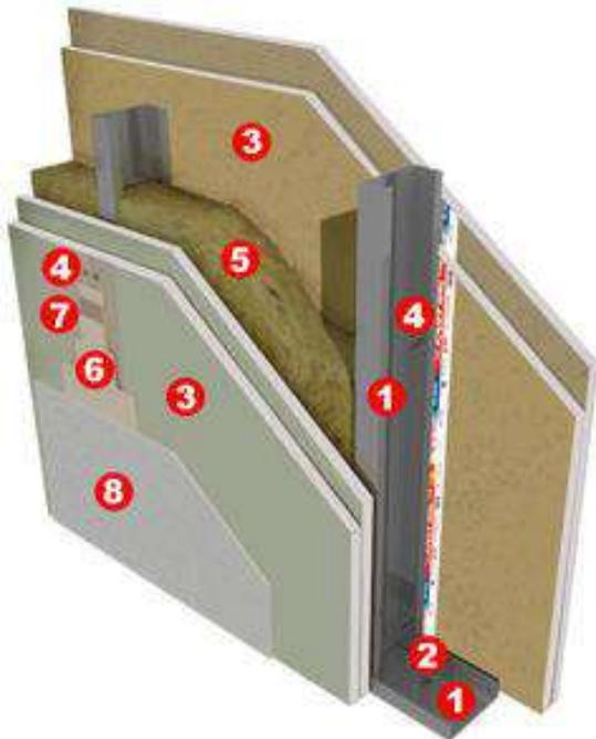
1. BASTIDOR METÁLICO CON POSTES 9.20 (3-5/8") A CADA 0.61 M.
